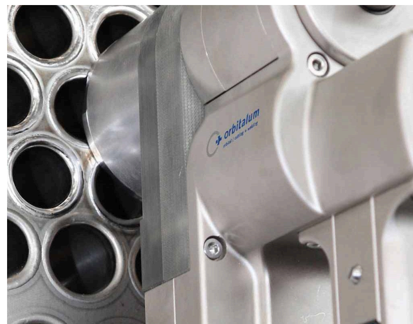
Tube-to-Tubesheet Orbital Weld Heads
